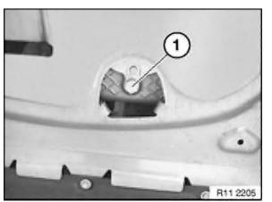
Open oil drain plug and drain off engine oil.
