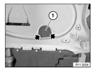
Drain or draw off engine oil. If engine oil is drained: **E46 only** Lever out cover (1) on side with a screwdriver.
